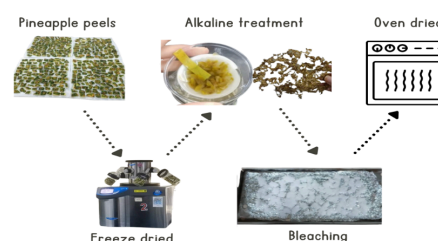
Fig. 1. Process for cellulose extraction from pineapple peel waste.
